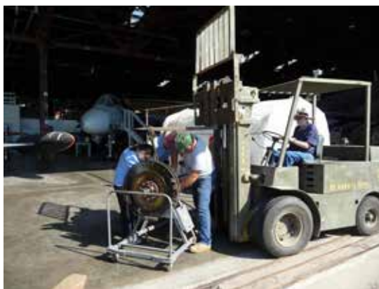
Below: Rachel Naylor, Danny San Romani, Gary Naylor and Don Dawson unload a J57 turbine wheel and shaft assembly Photos by Kevin Drewelow
